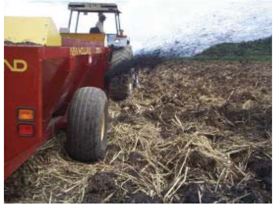
Fig. 5.11: Mud Spreader dispensing material up to band of 10m
